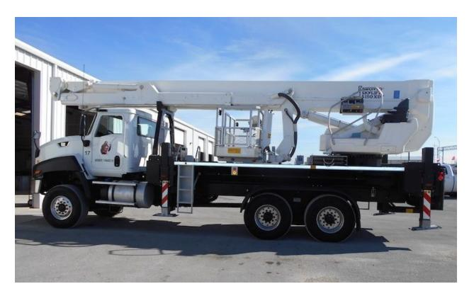
Some features of this model include robust Cat chassis, auto-leveling outriggers, 360° continuous rotation, a working platform of 3 ft x 7 ft with a basket capacity of 1,500 lbs, voice-in-command intercom, integrated in-basket water/electricity/air, and more.
